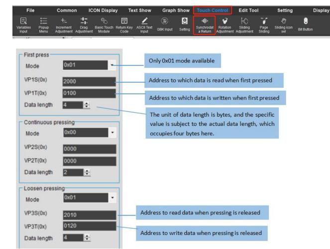
(4) Use the UE software to modify the 22 configuration file and cooperate with the synchronous data return control to realize the FSK bus camera.
