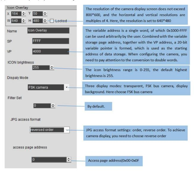
According to the T5L\_DGUS2 Application Development Guide, when the icon overlay control uses the bus camera display mode, it needs to reserve storage space backwards. Taking a display screen with a resolution of 640×480 as an example, 640×480÷8192=37.5 KB can be reserved as 40KB. The number of variable addresses occupied is 40×1024÷2=20480, which is 5000 in hexadecimal, and the following control variable addresses need to start from 0x9000.
