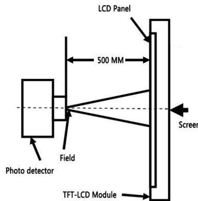
**Note 2: Definition of viewing angle range and measurement system.**
