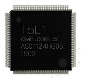
The T5L series ASIC is a single-chip and dual-core ASIC designed by DWIN technology co., ltd for AIOT applications with low power consumption, high cost performance, GUI and highly integrated application, including T5L1(low resolution) and T5L2(high resolution). Its main features are as follow:
