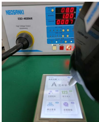
Electrostatic discharge test
