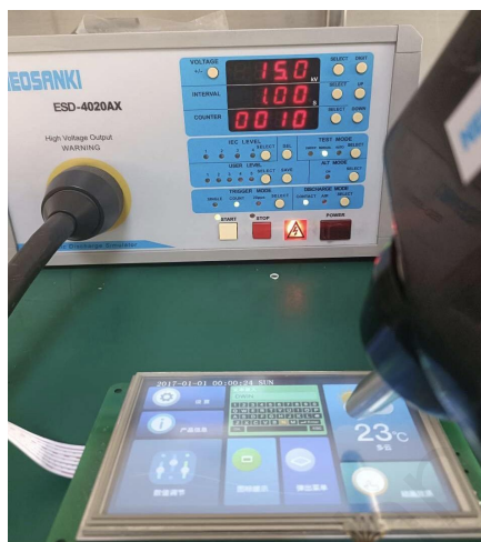
3.1 Electrostatic discharge test
