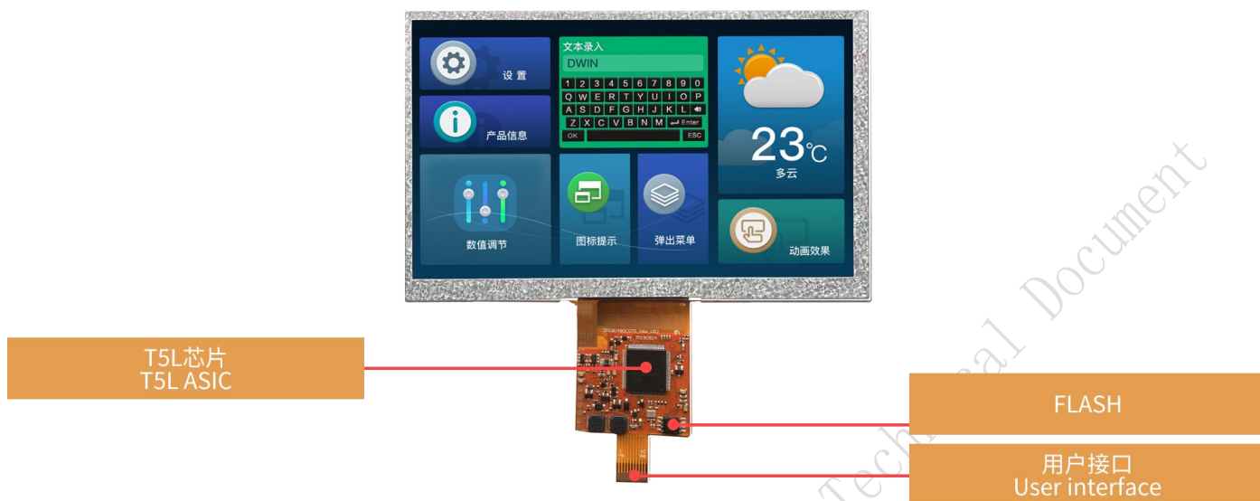
硬件接口图 Hardware interface
