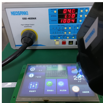
3.1 Electrostatic discharge test
