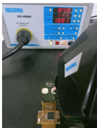
4.1 Electrostatic discharge test
