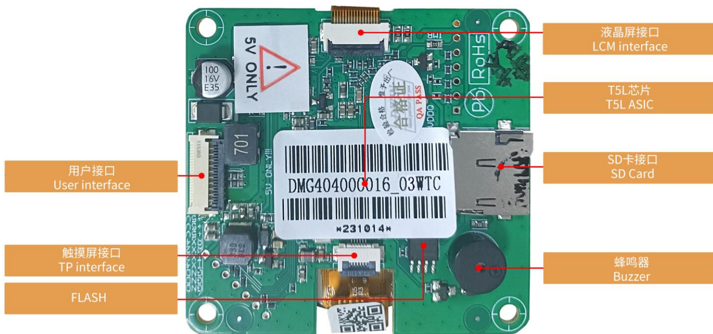
硬件接口图 Hardware interface
