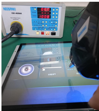
3.1 Electrostatic discharge test
