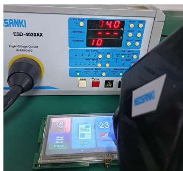
3.1 Electrostatic discharge test
