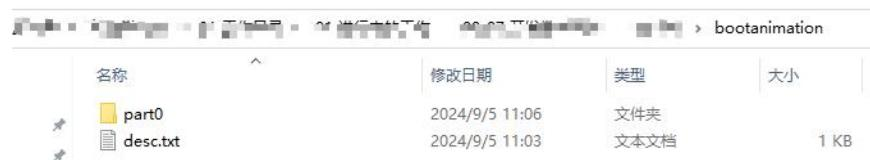
Create a new folder and name it as part0, put the animation pictures in it (.png format), naming pictures with 000.png, 0001.png, 0002.png and so on. Please note that the image resolution should not exceed the screen resolution, and the memory for a single image should be controlled within 2M. If the images are too large or too many, it may cause the startup animation to be unsMOOTHLY or freezed.
