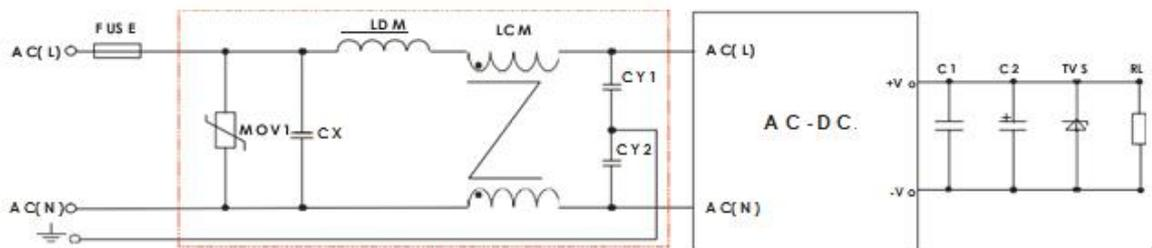
Note: EMC has higher requirements without any additional circuit.
